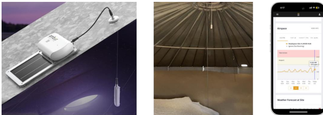
Figure 2. Monitoring stored grain using ACE AIR Analyzer sensor modules.
