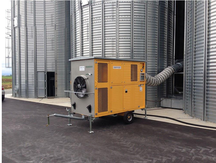
Figure 4.16. Chilled grain aeration system connected to the aeration ducting of an individual or set of steel silos. Mobile unit can be moved from silo to silo as well as along a warehouse and connect to aeration ducting to cool and maintain stored grain quality independent of ambient weather conditions.
