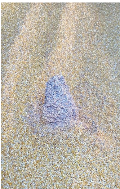
Figure 3.9. Evidence of the small amount of spoiled grain after some grain was removed from the silo after spiking CO 2 readings were observed in a silo over a one-month period indicating on-set of some spoilage and revealing the location of the small crack in the silo roof panel that allowed water to drip onto the grain surface whenever it rained. After the crack was properly repaired, the problem was eliminated.
