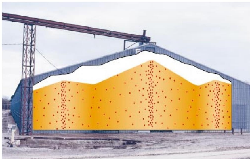
Figure 1.1. Illustration of spoutlines formed below drop points of three parallel overhead conveyors running the length of the warehouse filled with corn for longer-term storage. (Source: USGC)
