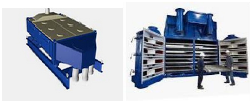
Figure 4.2. External and internal views of typical powered cleaners with multiple decks and replaceable screens of different sizes.
