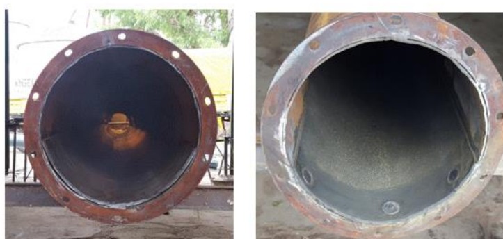
Figure 4.10. Examples of lining material installed inside downspouts to reduce additional corn breakage and wear of internal metal surfaces.
